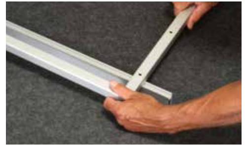
3. Place Channel underneath the frame, slide in hex nuts for assembly (add 2 extra and slide towards center for the Channel positions that are to be used for suspending the EchoSky)
