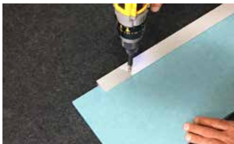
2. Place screw in pre-drilled hole of channel and fasten.
