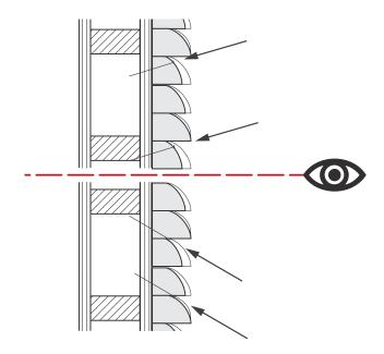
/ Where panels are to be installed onto a wooden backing surface, a tacker device may be used as an alternative (or in addition) to a polymer adhesive. For best results when using a tacker, take care to ensure that the appearance of the brads is minimised. When affixing wall panels above eye-level, brads should be 'shot' at a downwards angle. For panels below eye-level, shoot the brads at an upwards angle. Brads at eye-level should be shot into corners of the panel and between the lats.
