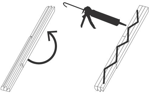
/ Panels may be mounted to a range of surfaces using the correct fixing medium and in most cases we recommend using a strong elastic MS polymer adhesive High Tech. As a guide, you will require roughly 290 ml adhesive for every 2 sqm of panelling.
