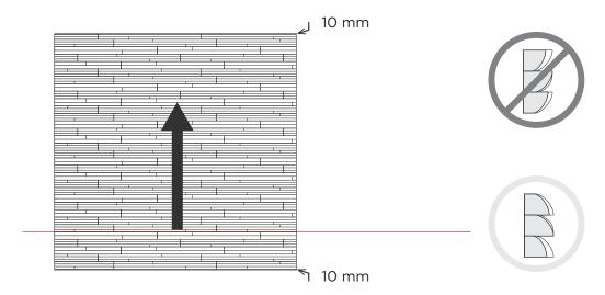
/ Place the panels in an irregular (mixed) formation and work first upwardly in rows until you come to the top of the wall. In each row, the leftover portion of panel from the end of one row may be used as the starting panel for the following row. Remember that this is subject to it's suitability to maintain the overall irregular formation; where it is not suitable, cutting to an alternative size should make it so. We advise leaving a 10 mm expansion space both below and atop of the wall.
