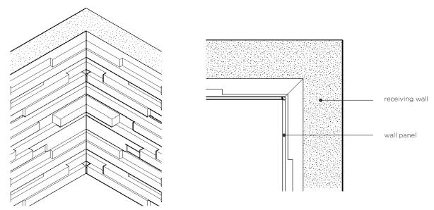
/ In case of an internal corner a seamless unbroken row of panels is achieved by joining corresponding panels using a mitered edge. Connect the return wall using the leftover piece from the joining panel.
