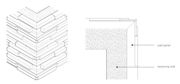
/ A seamless corner/unbroken row of panels is achieved by joining corresponding panels using a mitered edge. Connect the return wall using the leftover piece from the joining panel.
