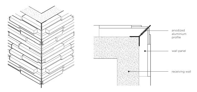
/ If a narrower, corner-defining solution is preferred we recommend using an anodised or powder coated aluminium profile of 4 mm thickness, positioned within the miter joint.
