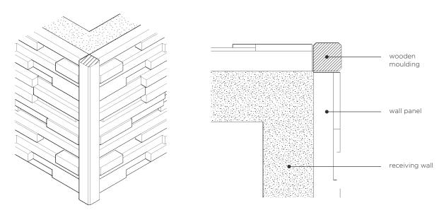
/ Using a square wooden moulding will delineate joining walls and put a strong emphasis on the corner itself. We recommend that you use a well matched wood type for this solution.
