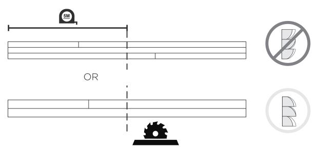
/ For the most efficient coverage, cut the first panel directly in half, widthways (with a tablesaw or a cross-cut saw). Taking one of the resultant half panels, align the newly created straight edge with the left edge of the wall and fix in place. Gallon has two types of panels, one divided in two strips and the other type divided in three strips (as shown in the image above). Make sure you finish each row with the same type of Gallon panel and that the lamellas are oriented downwards.
