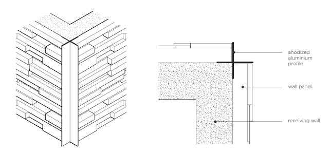
/ For this open corner solution we recommend using an anodised or powder coated aluminium profile of 50x50 mm.
